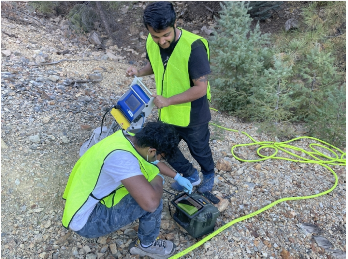
Team members led by ASU Assistant Professor Hamed Khodadadi Tirkolaei measure dust generation from the surface of a mine waste deposit at the abandoned Cash Mine near Prescott, Arizona, after applying enzyme-induced carbonate precipitation to stabilize the surface. Photo courtesy of Hamed Khodadadi Tirkolaei
