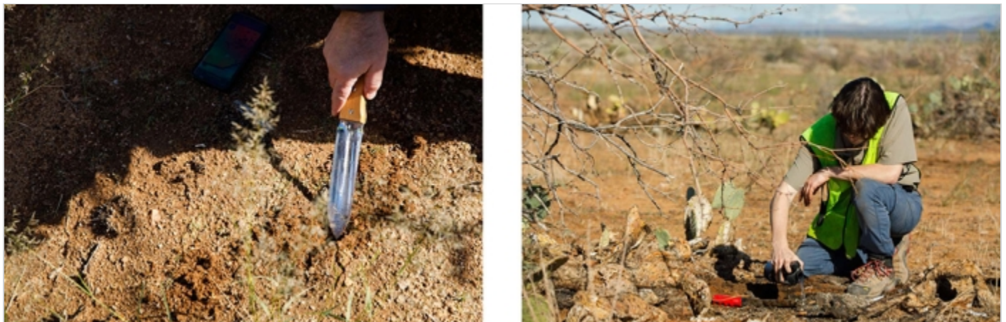
A soil knife (a skinny shovel with measurement markings engraved on it), water bottle, soil condition guide and smartphone camera were the only tools they needed to “field truth” categories of low, moderate and severe burns at the Saddlebrooke Fire. Martin and the other researchers measured plant cover, ash depth, soil structure, surviving roots and how quickly water infiltrated the soil. Photos by Andy DeLisle/ASU
