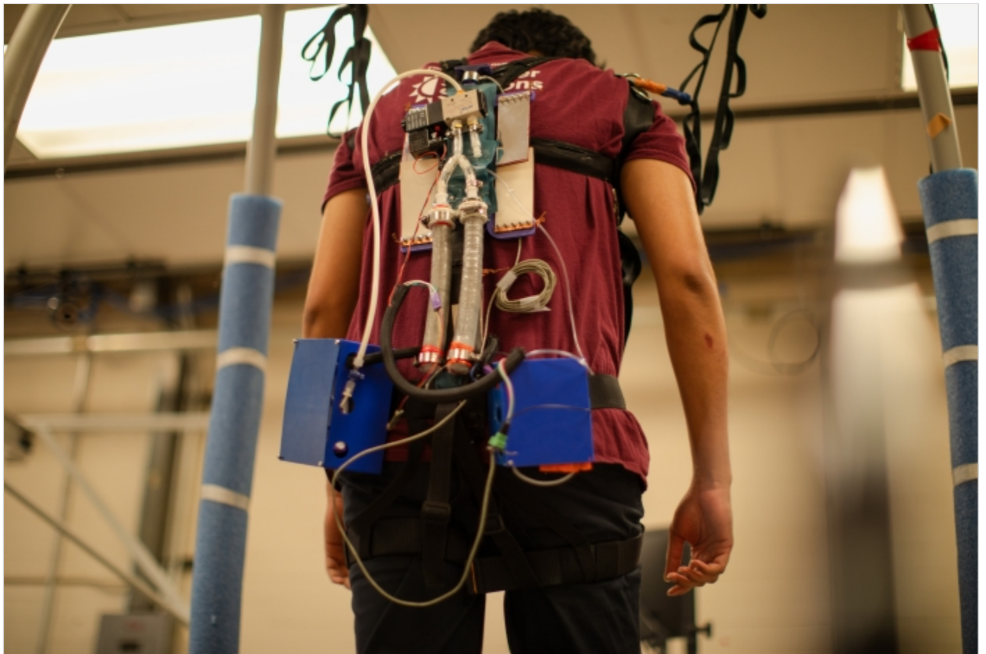
Mechanical engineering doctoral student Rohan Khatavkar does a treadmill test on the back support device his team designed in the Robotic Actuators and Dynamics Lab. Photo by Samantha Chow/ASU
