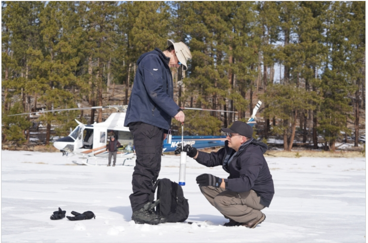
SRP meteorologists Bo Svoma (left) and Matthew Pace measure snow depth and density along a snow transect near Hannagan Meadows SNOTEL (SNOWpackTELEmetryNetwork) station.
