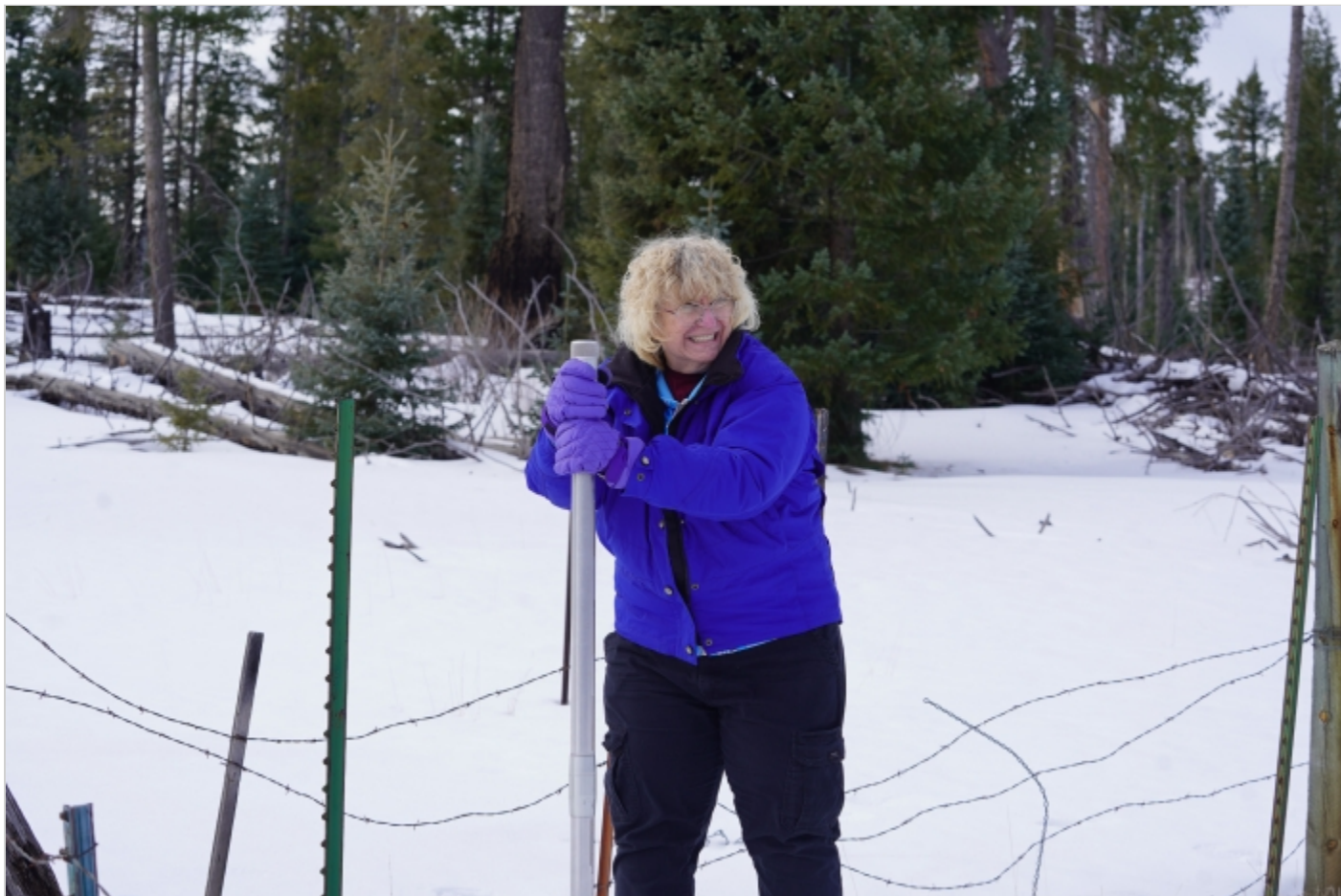
Valerie Swick, water resources planner with the U.S. Bureau of Reclamation, measures snow depth and density at Hannagan Meadows SNOTEL (SNOWpackTElemetryNetwork) station.
