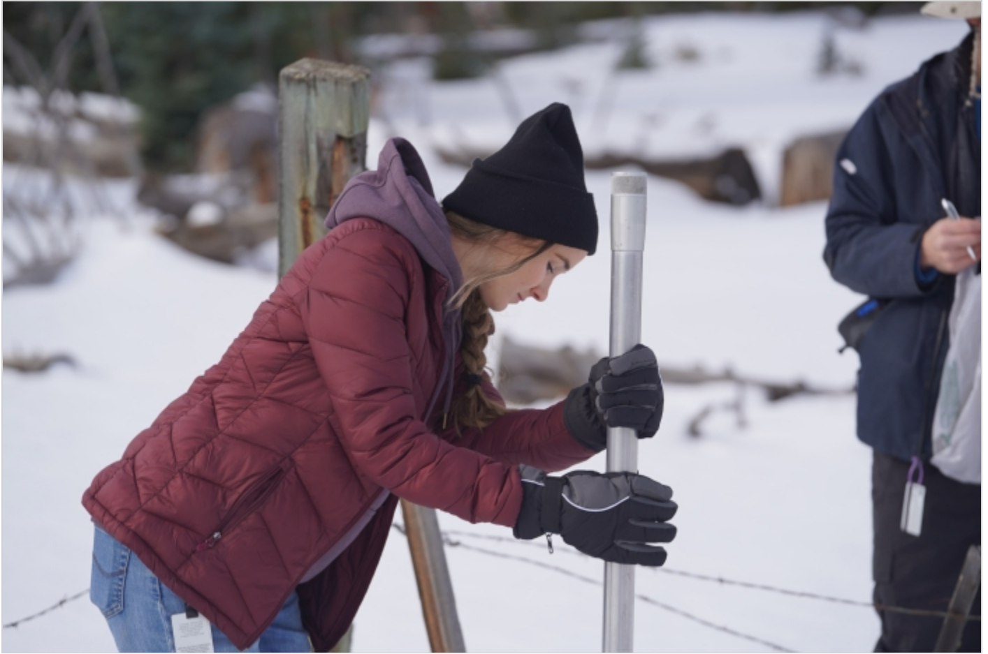
SRP meteorologist Jessica Moeschl measuring snow depth and density along a snow transect near Hannagan Meadows SNOTEL (SNOWpackTElemetryNetwork) station.
