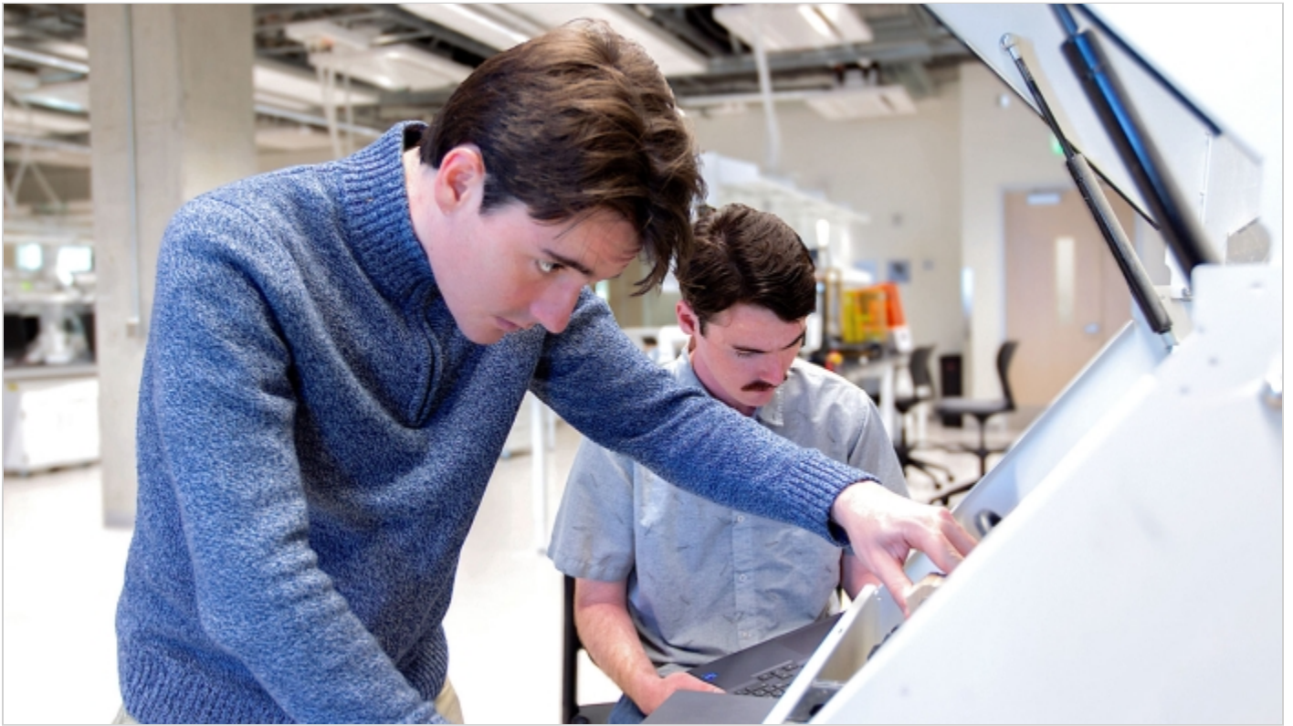
Cameron Peavy (left) and Aaron Peavy, manufacturing engineering undergraduate students in the School of Manufacturing Systems and Networks, set up a wooden part in the Penta 5 Axis CNC machine in the Robotics Systems Instructional Lab, located in ISTB 12 on ASU's Polytechnic campus. Photo by Aisha Kaddi/ASU
