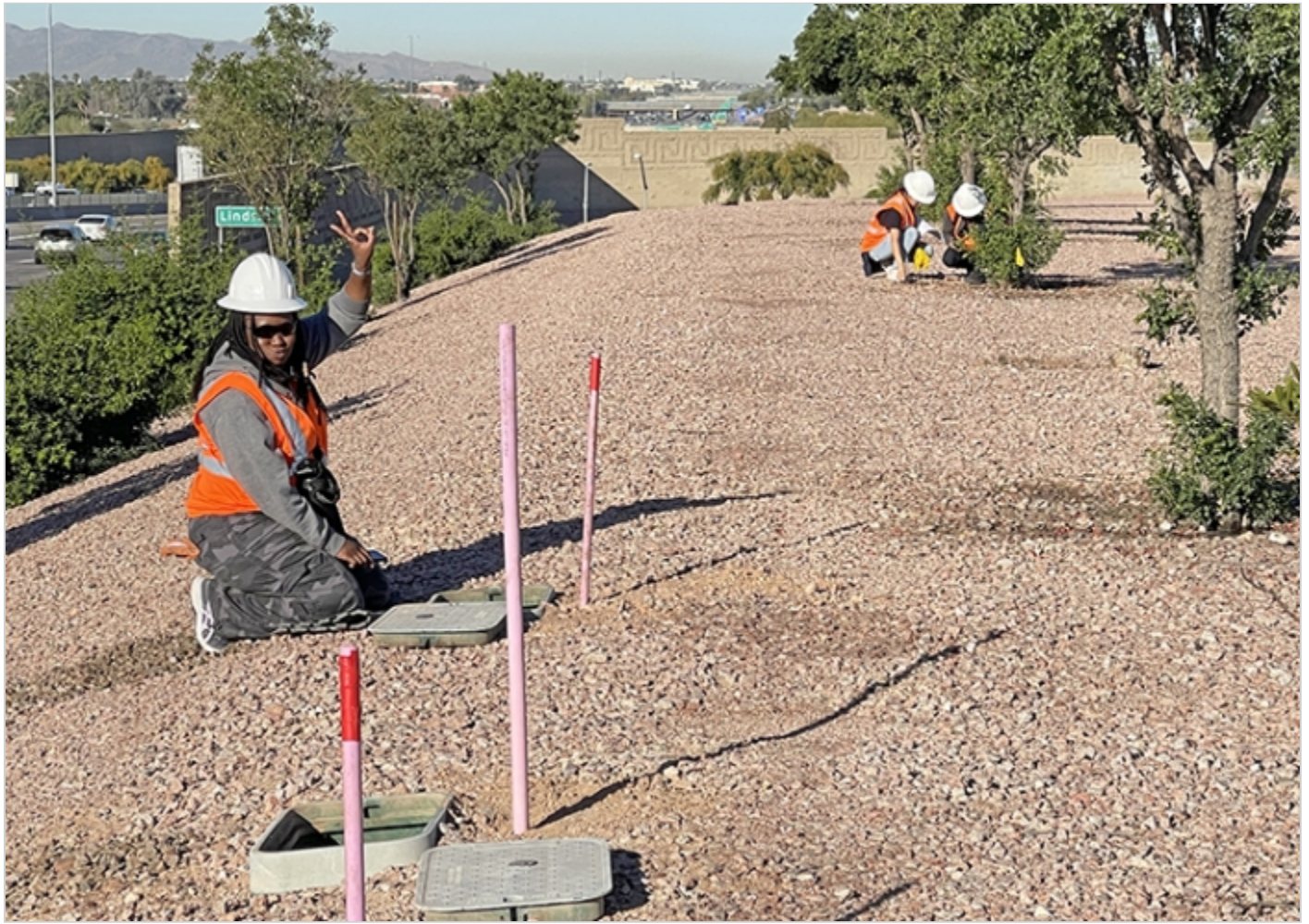
Student researchers collecting pressure data (foreground) and emitter performance data (background). Photo by Harry Cooper/ASU
