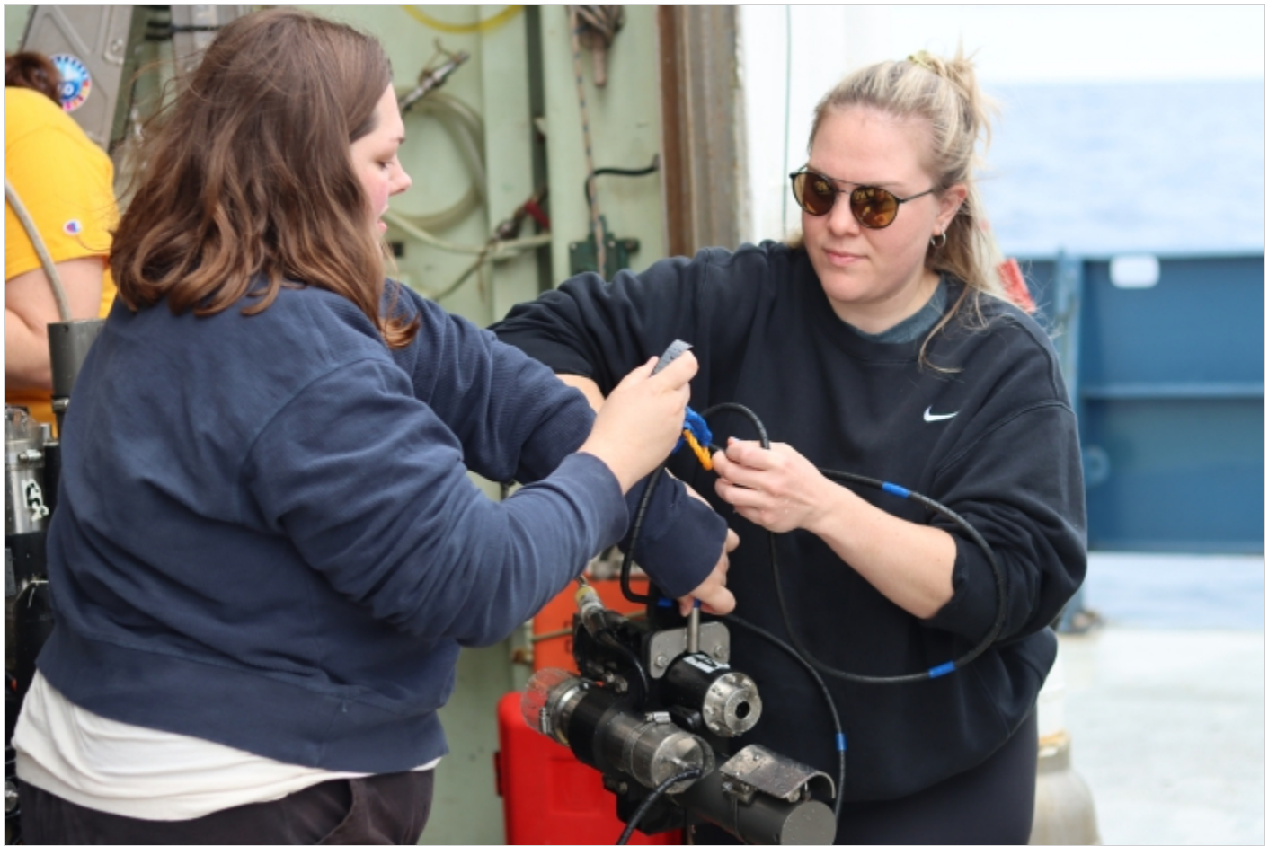
Isobaric gas-tight samplers are carefully retrieved from Alvin's basket for processing and analysis.
