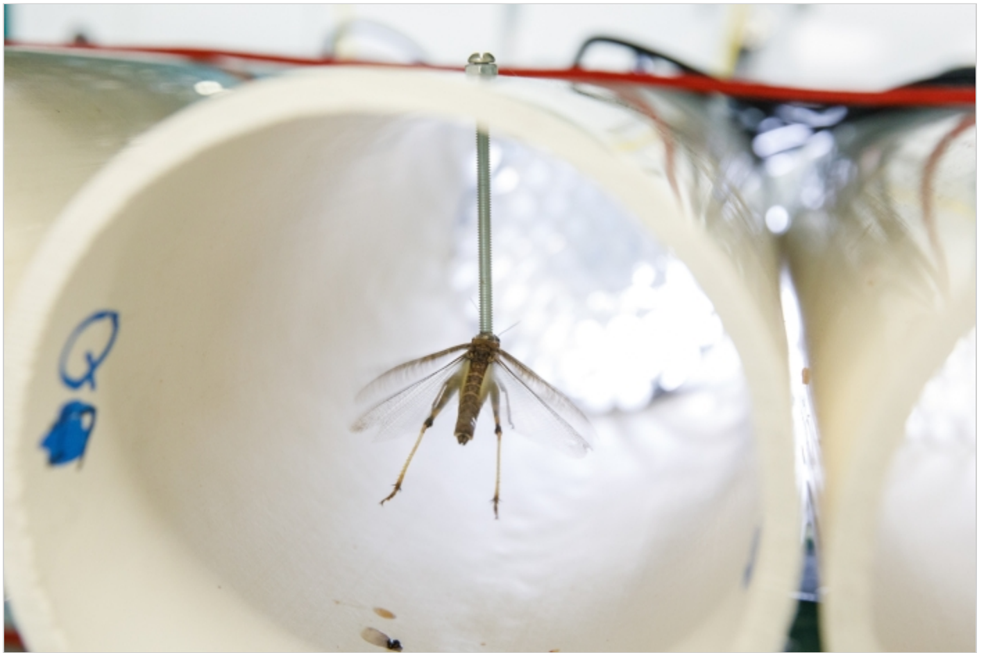
A locust (held in place thanks to a tiny magnet) flies in a wind tunnel to measure its flight duration. It's the insect's version of running on a treadmill. Photo by Quinton Kendall/ASU
