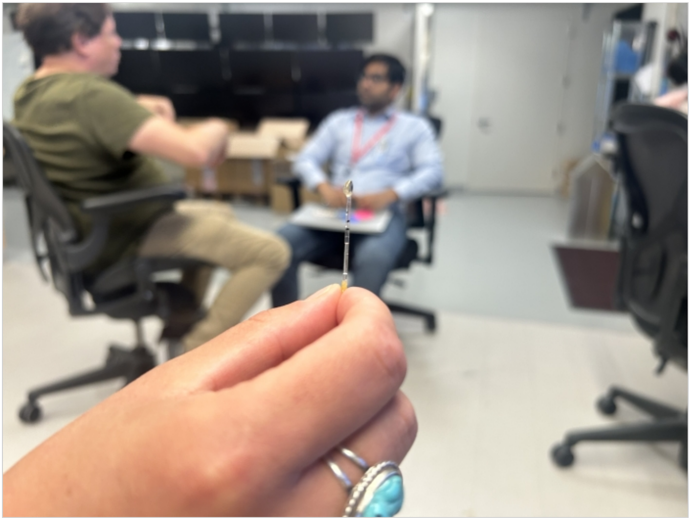
Sabine Botha shows the 1-millimeter-width microcuvette that will hold the first protein sample (proteinase K) to be placed in front of the X-ray beam.
