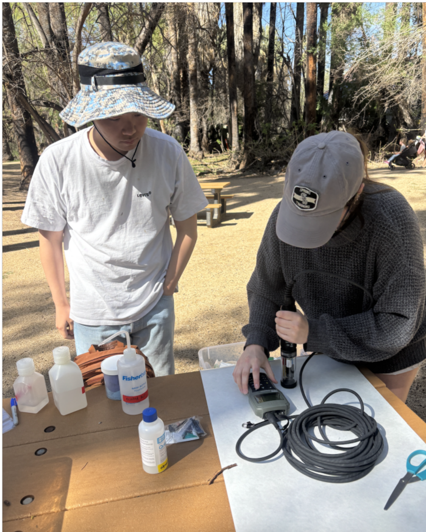
Weiyu Wu and Paige Sturm calibrate the dissolved oxygen probe at the Hassayampa River Preserve.
