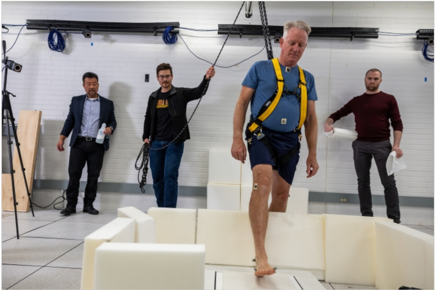
Small reflective spheres mark hips, knees and other major joints as volunteers step onto a slippery surface inside a simulated bathtub. Foam sides are used instead of an actual bathtub in order to protect volunteers from injury when their feet and legs strike the edges.
