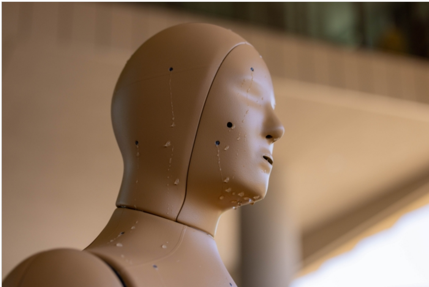
ANDI, the world's first indoor-outdoor breathing, sweating and walking thermal manikin, sweats while out on campus in August. The manikin will help researchers better understand how different human bodies with different health situations are impacted by heat stress. Photo by Samantha Chow/ASU
